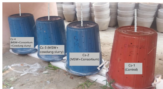
Fig. 1 Experimental setup of passive aerobic bin composting
