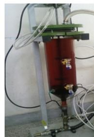
**Figure 1** Biodiesel production from transesterification method.
